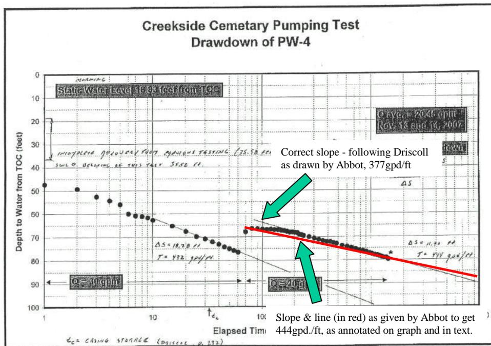
Abbott's figure "Pumping test drawdown of PW-4" (ASE Appendix B, 2008), there is a line through the points from about  $t=200$  minutes to  $t=1440$  minutes. If you use this line to calculate  $T$  you get a drawdown of 68 feet at 200 minutes and a drawdown of 82 feet at 2000 minutes, which gives  $\Delta s$  of 14 ft and  $Q = 20$  gpm. Then applying the formula  $T = 264 Q / \Delta s$  (Driscoll p. 221, equation 9.7) gives  $T = 264 * 20 \text{ gpm} / 14 \text{ ft} = 377 \text{ gpd/ft}$ .
