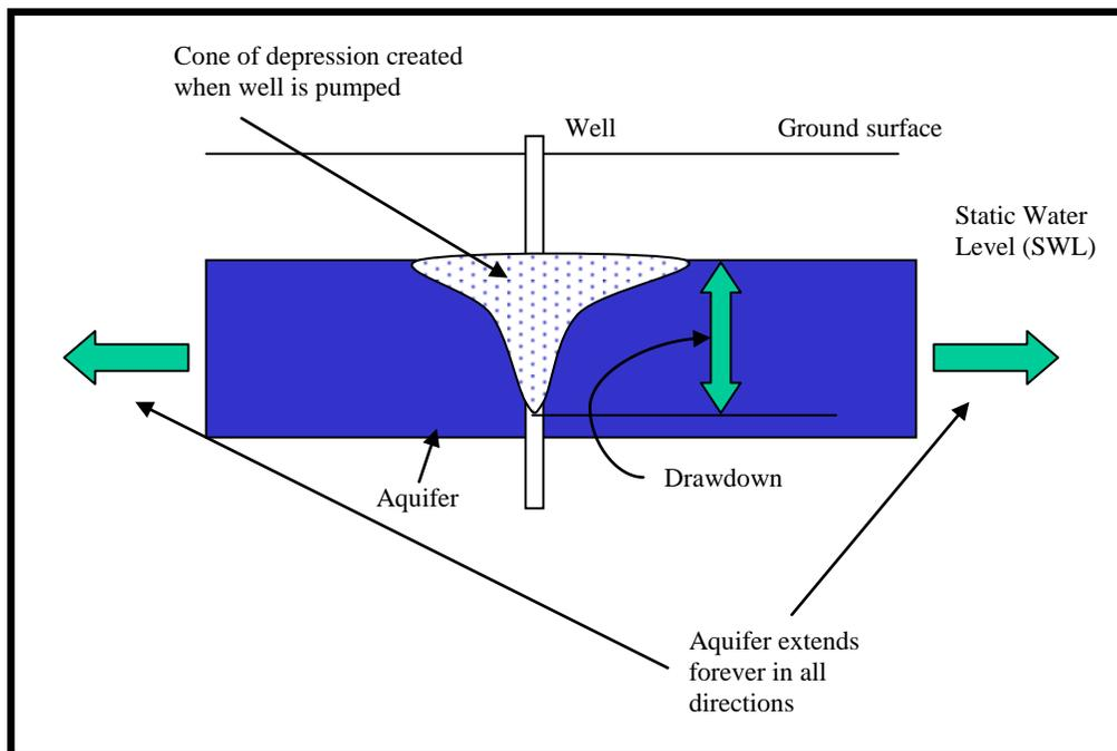
When the aquifer is larger than the cone of depression, then the cone of depression will expand in a way that can be predicted by the modified non-equilibrium well equations (Driscoll p. 219). When the well drawdown level is plotted versus time on a logarithmic scale, the result is a straight line (Driscoll, p. 220, figure 9.13).
